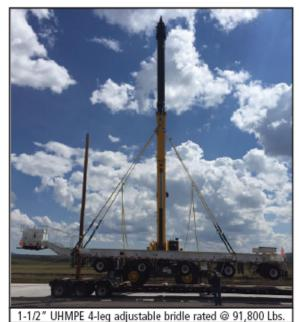
Lift-It• Three and Four Leg PROLINE12<sub>TM</sub> UHMPE Adjustable Rope Slings feature a Top Lifting Link. Depending upon your selection, based on Work Load, you must determine whether a Masterlink or Masterlink with Subassemblies makes the most sense from a fitting weight perspective. With either option, heavy duty thimbles are attached at the connection points to the Top Lifting Link.
